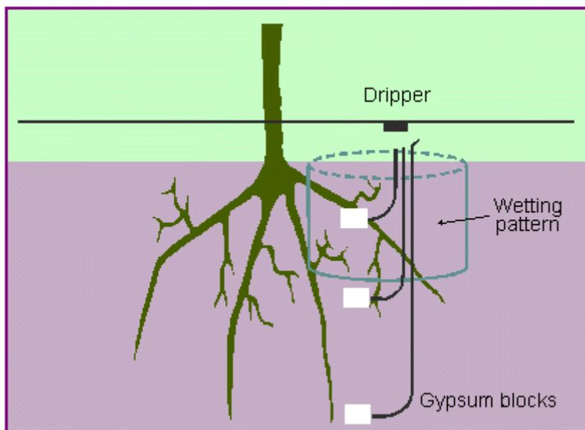
*Recommended placement of gypsum block in relation to the emitter, the wetting pattern and the root distribution under a vine (from P.D. Mitchell and I. Goodwin, Micro Irrigation of vines and fruit trees, Agriculture Victoria, 1996, Agmedia).*
