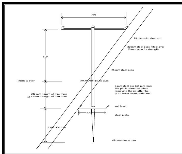
**Figure 5: Use of Jig to construct Tatura Trellis.**
