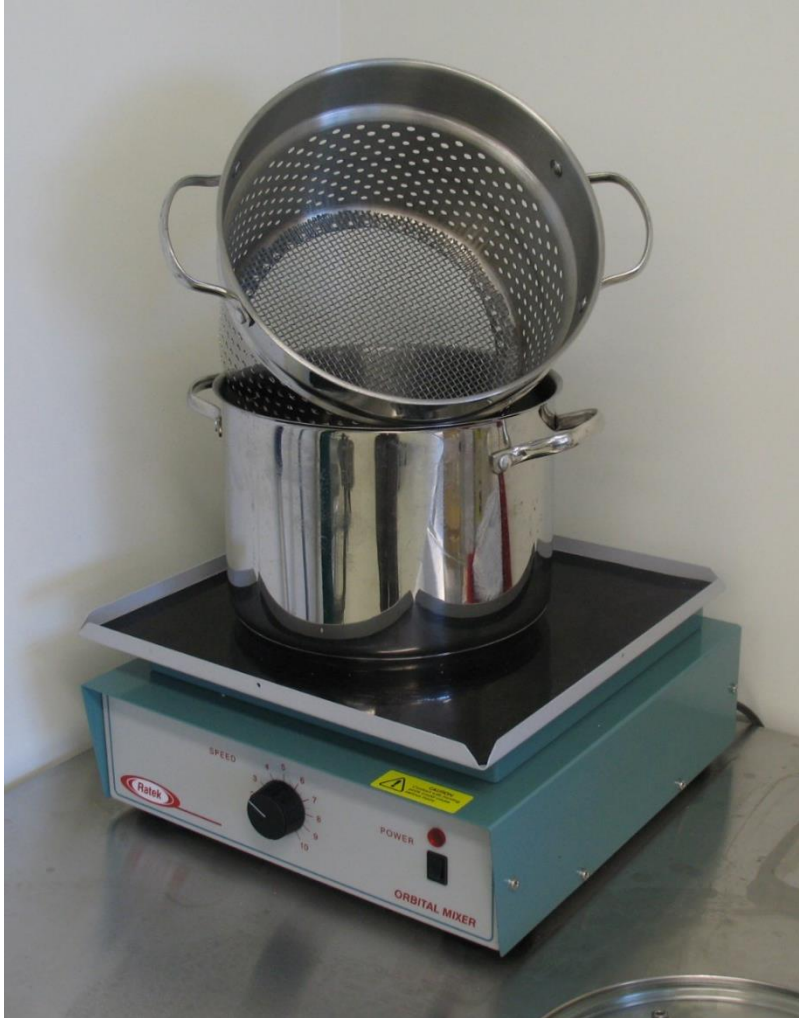
Figure 1 Bee 'shaker' used to screen swarms for mites
