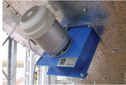
Aeration fans fitted to silos can rapidly reduce grain temperatures
