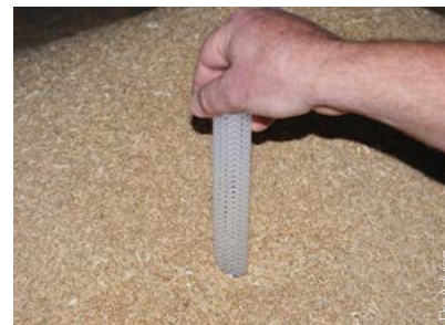
Probe traps pushed into grain at the top of silos or bulk grain storages help detect the first signs of an insect infestation
