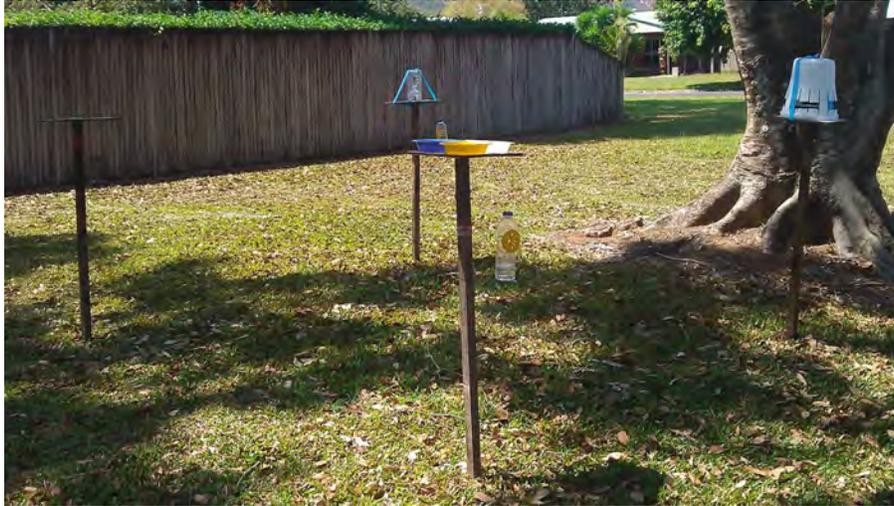
**Figure 2:** Setup of timber platform stations and traps during efficacy field trials; traps were randomly placed on or hung from timber stations placed at the corners of a 2 x 2 m square. Clockwise from left: sticky mat trap, pheromone trap & artificial flower bottle trap; AHB trap; pan traps & artificial flower bottle trap.
