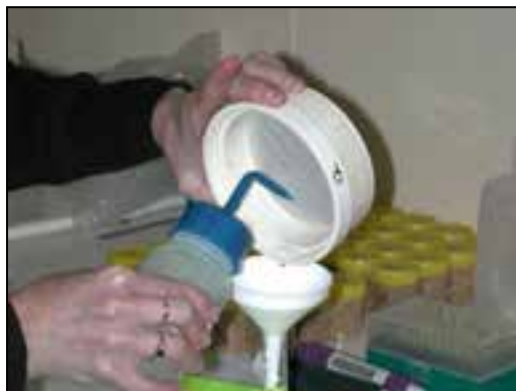
Figure 2.3 Washing the deposit from the 15-µm sieve into the centrifuge tube.
