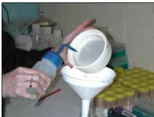
Figure 2.2 Washing the deposit on the membrane to one side of the 15-µm sieve.
