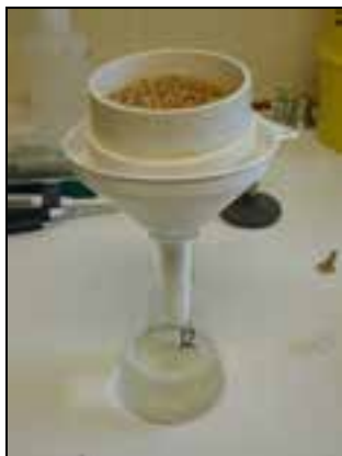
Figure 2.1 The set up for the selective sieve wash test. Two sieves (50 µm and 15 µm) are placed within funnel on top of the 500 mL Erlenmeyer flask.
