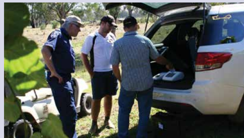
Instead of a laboratory, LAMP allows samples to be tested for particular bacterial infections in the back of a car. Image courtesy of Plant Biosecurity CRC
