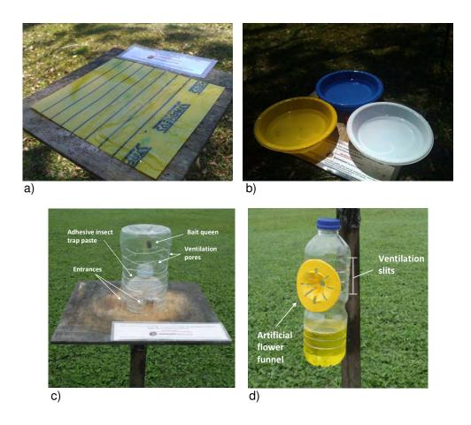
Figure 1: The experimental traps used during efficacy field trials: a) sticky mat trap; b) pan traps; c) pheromone trap; d) artificial flower bottle trap
